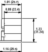
NOTE: SMALL MOUNTING HOLES FOR SELF THREADING #4 SCREW. LARGE MOUNTING HOLES FOR #8 SCREW 0.95 (24.1)
