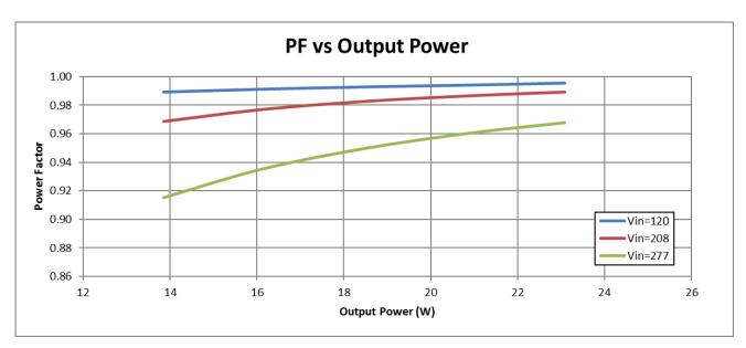
Output power based on maximum rated output current and varying load voltages.
